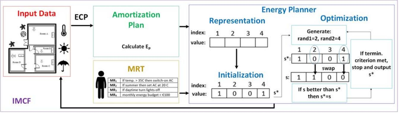
Fig. 4. Example execution of the IMCF framework Planner.
